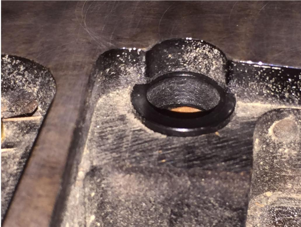
You may need to tap the ring in, especially for the last few millimeters. When the gap noted in step 8 is gone, stop! If you try to go beyond this, you can damage the face of your guitar.
