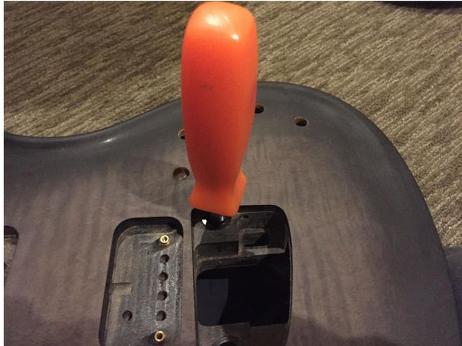
10. After removing the bushings, find the depth of each bushing hole. I used a folded up piece of paper inserted into the holes and marked the back edge of the body.
