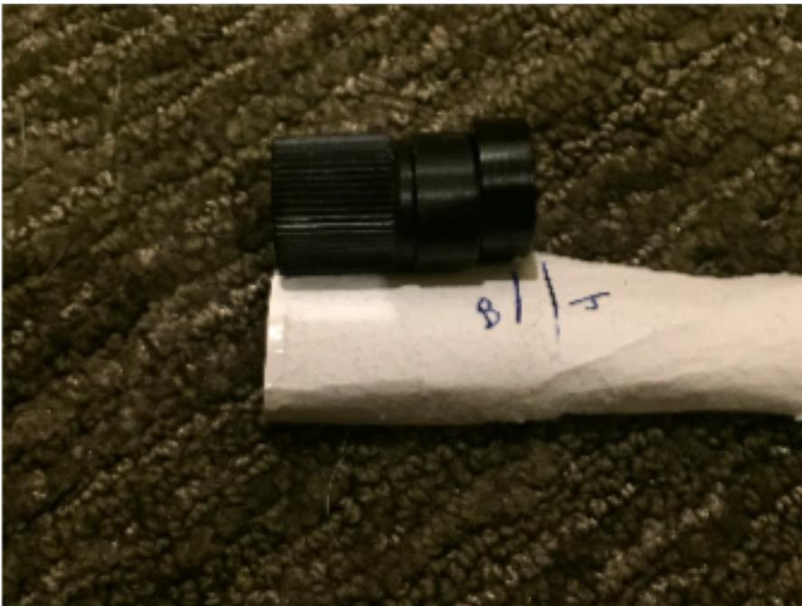
If the ring plus bushing is thicker than this measurement (as shown on the bass side), you'll need to sand the ring down using some sandpaper until it is the required thickness. Otherwise, your bushing will stick out the back of the guitar and the cover plate won't fit.
