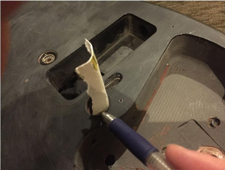
11. This will help you figure out the thickness that the plastic ring needs to be for a perfect fit. If it is already the correct thickness or a little smaller, go to the next step.
