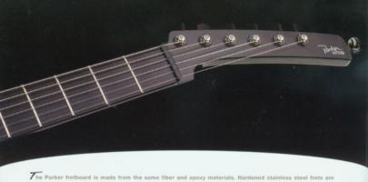
The Parker fretboard is made from the same fiber and epoxy materials. Hardened stainless steel frets are bonded to the fretboard surface with a tough adhesive. This patented process creates a perfect fret job. Our slippery frets seriously outwear other frets and don't require the frequent fret leveling needed on conventional guitars. The Parker Fly's lightweight truss rod (only 1/6th the weight of conventional rods) easily adjusts the neck to accommodate string gauges, handling .008s to .013s.
