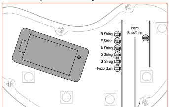
We set these controls at the factory so that the individual string piezo outputs are balanced and the full volume outputs of the piezo and magnetic systems are equal.
