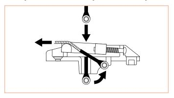
Intonation is a subtle string-length adjustment that tunes the string to the fretboard. Intonation adjustments can be made by adjusting the intonation screws at the rear of each saddle clockwise to move the saddle back (to make the string play more flat), and counterclockwise to move the saddle forward (to make the string play more sharp).
